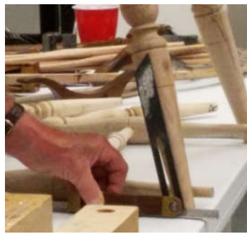
USING A BEVEL SQUARE TO DETERMINE THE ANGLE TO DRILL THE LEG HOLES FOR THE STRETCHERS
