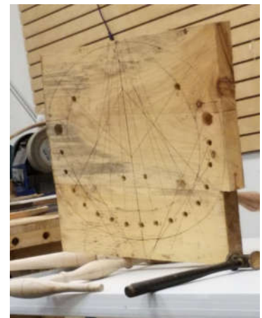
SEAT BLANK SHOWING SIGHT LINES TO DRILL HOLES FOR SPINDLES, LEGS AND ARM SUPPORTS
