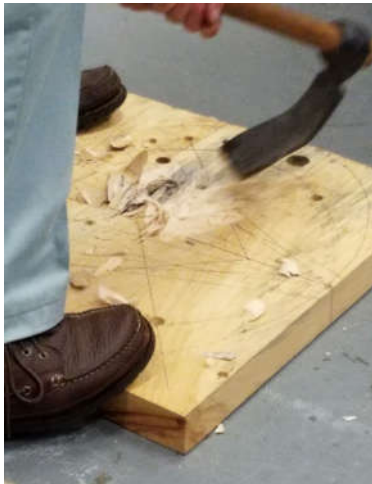
ROUGH FORMING THE SEAT USING A GUTTER ADZ
