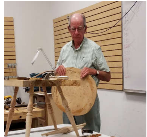
THE PLYWOOD PATTERN WHICH DESCRIBES THE LOCATION OF THE PARTS ON THE SEAT
