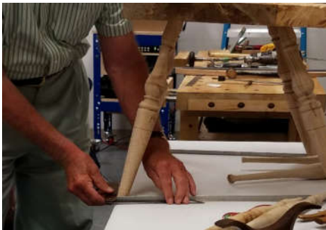
USING A BEVEL SQUARE TO DETERMINE THE ANGLE TO DRILL THE LEG HOLES FOR THE STRETCHERS
