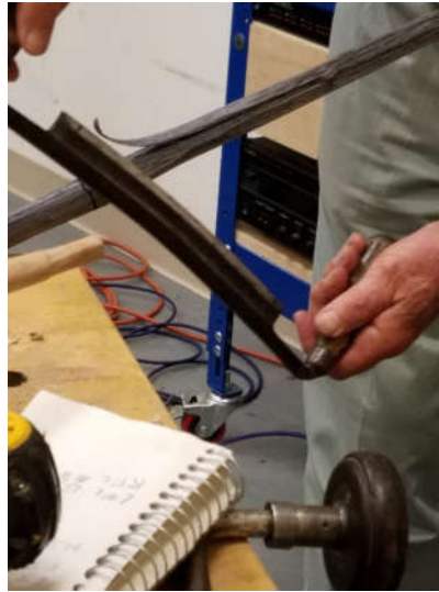
FORMING A SPINDLE USING A DRAWKNIFE
