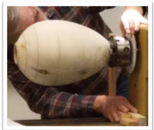
-Drawing radial and segment lines using a pencil holder to draw the lines - see photo below
