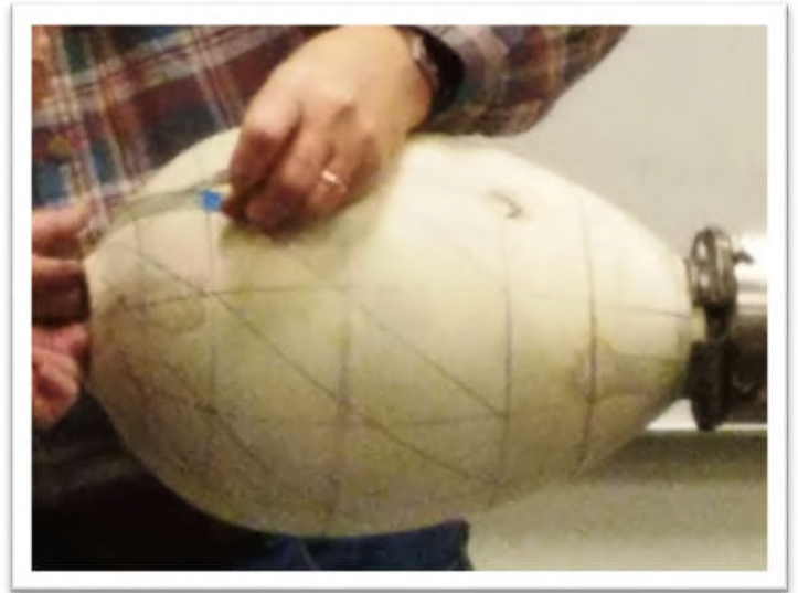
Drawing the spirals - using flexible pieces of thin plastic to draw the lines
