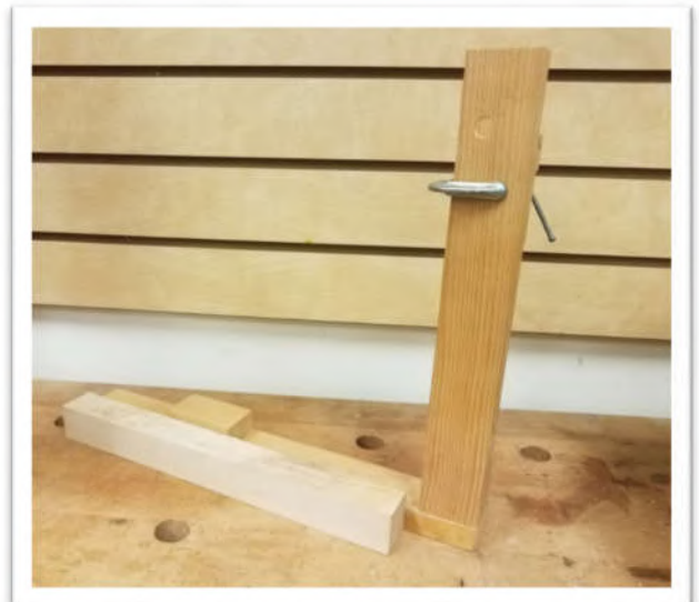
Jig to hold pencil for drawing radial and segment lines – see photo above
