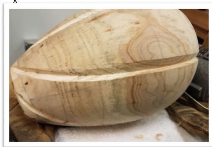
V-grooves are completed ready to be smoothed with planes, rasps and/or files
