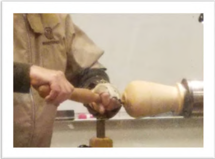
Parts of sides, #2 and #3 on hollowing chart are removed with the angled or shoulder cut tool
